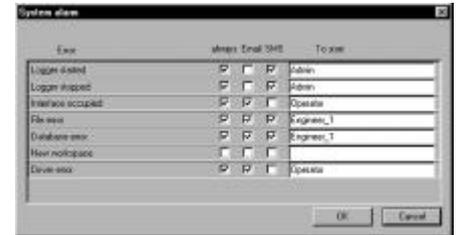
All system events are logged in an alarm log. The user logged on the moment the alarm is received can view the log and acknowledge alarms. The alarms can be acknowledged individually or all at once. Depending on the setting either all alarms or only unacknowledged ones are displayed.
